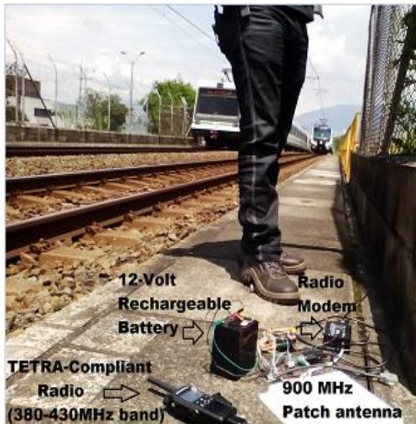
Figure 13. On-the-field tests to verify communications of network node prototype with the ground station
