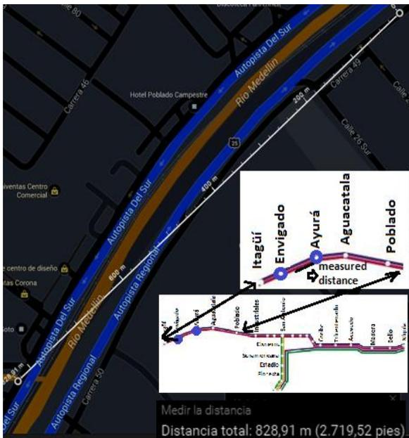
**Figure 11. Distance to be covered between the site and the ground station**
