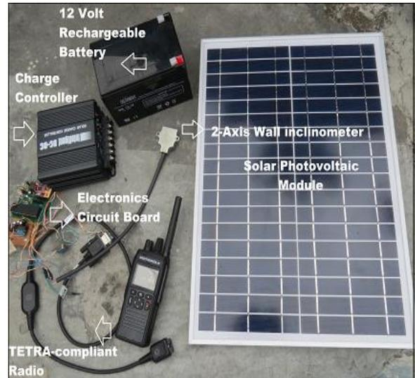
Figure 15. Basic set of elements to start on-the-field continuous operation test in order to validate prototypes
